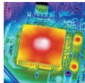
Printed circuit heat buildup
